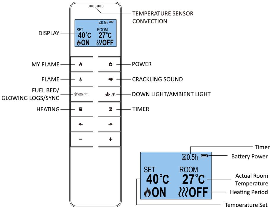
**NOTE: The remote control handset must be left in the same room as the appliance because it houses the thermostat that regulates heat output. Also, when using the APP, the remote must also be in same room and have batteries fitted and working to ensure accurate temperature control.**
