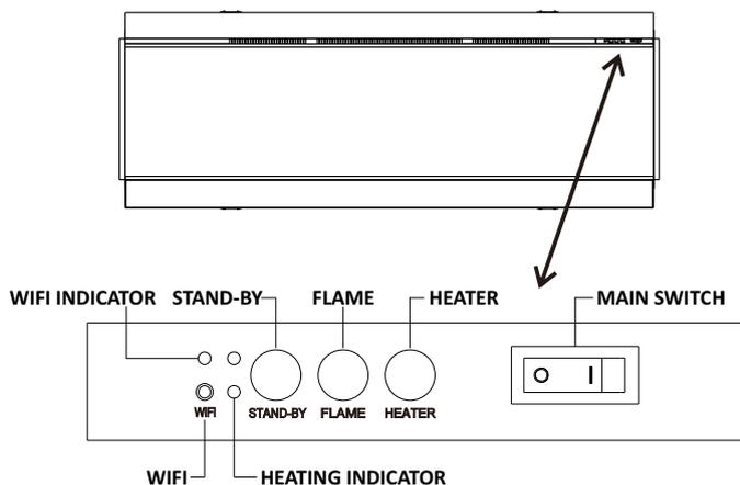
Each time a button is pressed on the appliance or on the remote control, an audible beep is emitted. To turn off this feature, keep pressing button **FLAME** for 3 seconds until you hear two beeps.
